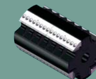
CHIPPER ROTOR-4 POCKET with four rows of knives for chip lengths of 1/16" to 1/2"; to produce short chips from stem wood suitable for pelletizing or pulverized fuel, etc.
