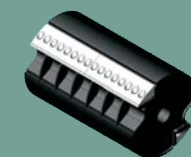
CHIPPER ROTOR-2 POCKET with two rows of knives for chip lengths of 3/4" to 1-1/4"; to produce fuel chips from stem wood
