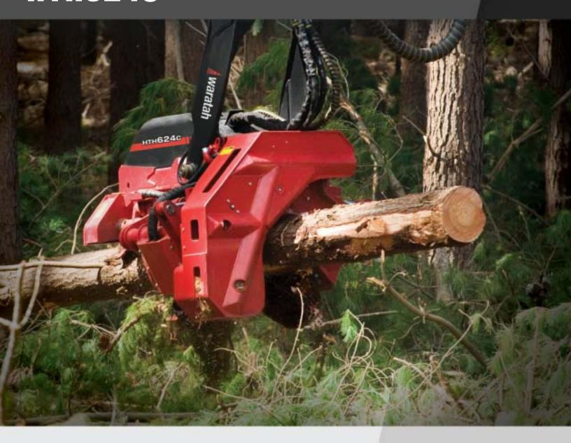
Proven in medium to large wood harvesting and processing, Waratah's big-timber-tackling HTH624C can easily handle species such as radiata pine, poplar, and aspen — up to 81 centimeters (32 inches) in diameter. With its rugged frame, large synchronized feed rollers, incredible drive power, and precision delimbing quality, it's a highly productive processor — whether you're working at a landing or felling and processing at the stump.
