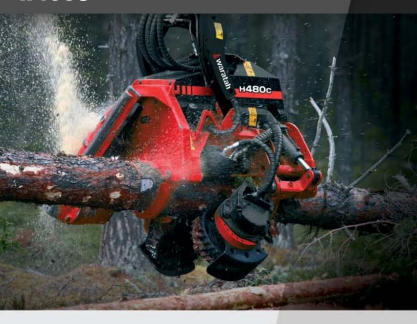
The Waratah H480C harvesting head combines large timber cutting-power with an excellent delimbing quality throughout its diameter range.
