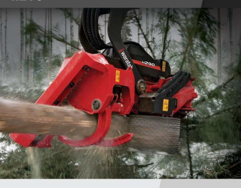
The Waratah H290 is a powerful, high-capacity new-generation harvester head. Built for superior performance in regeneration harvesting, it was specially designed for use with large wheel- and track-based harvesters.
